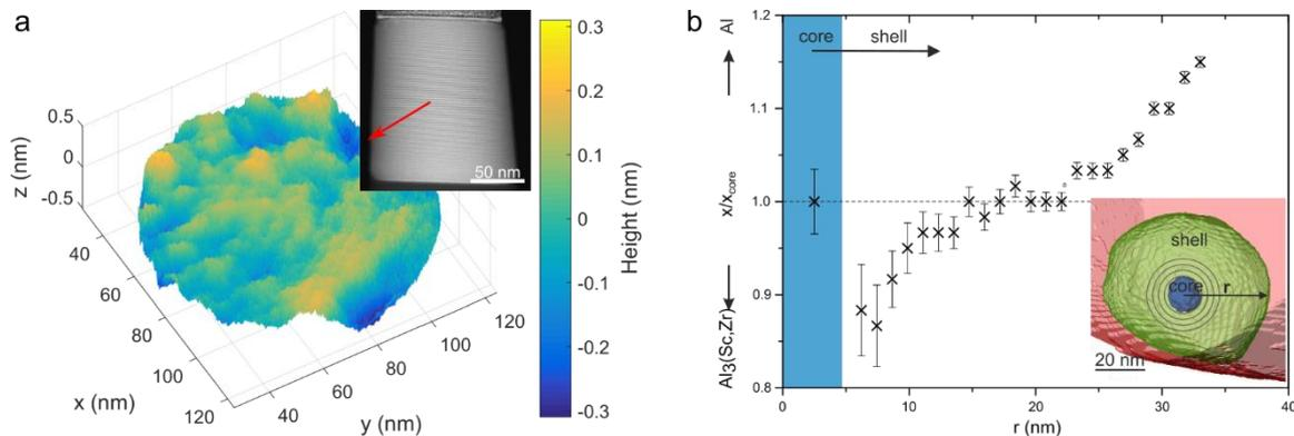
**Figure 1.** (a) ADF STEM projection of a Mo/B<sub>4</sub>C multilayer (inset) and reconstruction of one interface within the multilayer. (b) Changes of Al content in a core/shell particle within an Al-Mg-Sc-Zr alloy.
