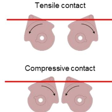
**Figure 2.** Working principle of the rotational sample clamps. Other clamp designs available.
