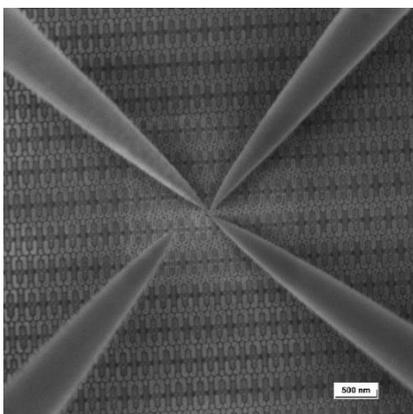
**Figure 3.** 500 eV SEM image of SRAM cells with nanoprobes landed on the bit-cell contacts (Scale of 500 nm)
