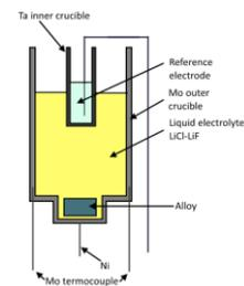
Fig. 4 Illustration of cell for EMF measurements
