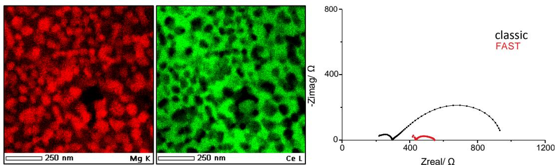
**Figure 1.** High-resolution TEM images of the composite samples. **Figure 2.** Nyquist plots of the impedance spectra of FAST and classically sintered samples at 540 °C.
