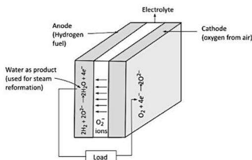
Fig.1. A single cell in a SOFC fueled with hydrogen [2].
