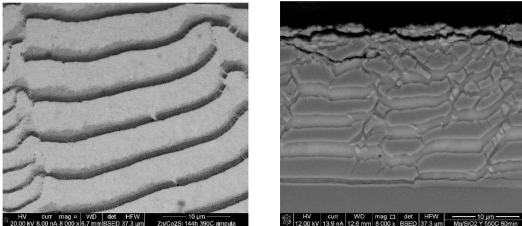
**Figure 1.** The microstructures of the periodic patterns formed in Zn/Co<sub>2</sub>Si (left) and Mg/SiO<sub>2</sub> (right) diffusion couples.
