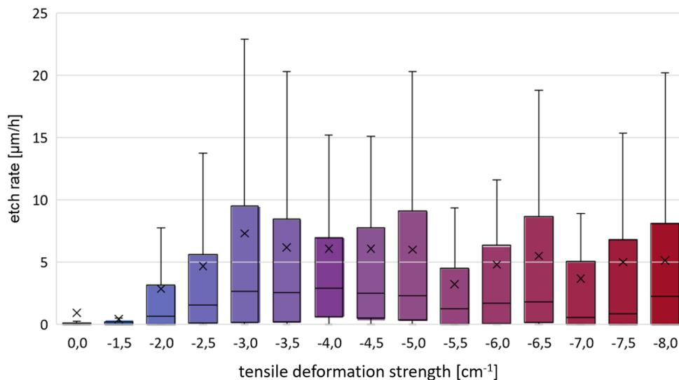
**Figure 1.** The correlation between the acidic etch rate and the deformation strength of tensile strained silicon on mechanical and thermal treated samples.
