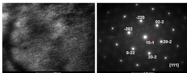
Figure 1. TEM/ DF Coherent Ni<sub>3</sub>Al type precipitates, annealed for 0.5 h at 973K.
