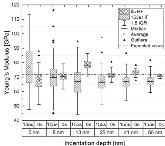
**Figure 1.** Young's modulus measurement statistics on Fused Silica after HF-etching at several indentation depths. With higher surface roughness and lower indentation depths, the scatter of the data increases. The Young's modulus values of the rough sample (155s HF) tend to be underestimated.
