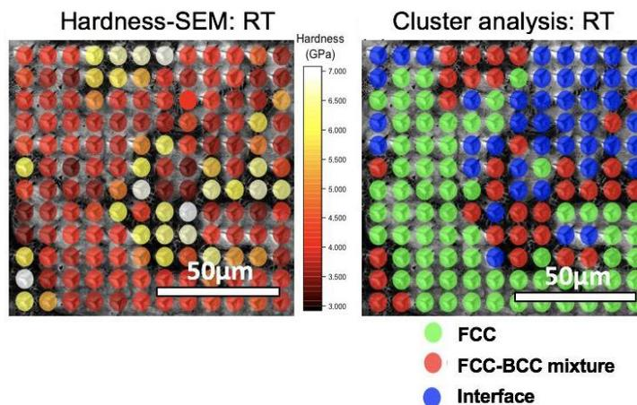
**Figure 1.** Hardness of HEA with Al of  $x=0.3$  overlaid on SE micrograph. Normalized hardness and modulus used as clustering parameters to produce cluster overlay from same dataset.
