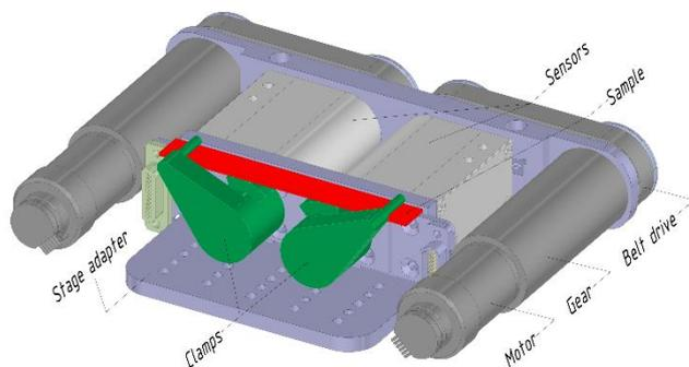
**Figure 1.** CAD drawing of the in-situ 4PB device.
