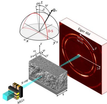
**Figure 1.** A schematic drawing of the CSnanoXRD setup. The experiments are performed in transmission diffraction geometry, where thin film lamella with a width of  $L$  is exposed to a X-ray nanobeam focused by crossed multilayer Laue lenses (MLLs). The specimen is moved along the  $z$  axis and diffraction data are collected using the Eiger X 4M 2D detector.
