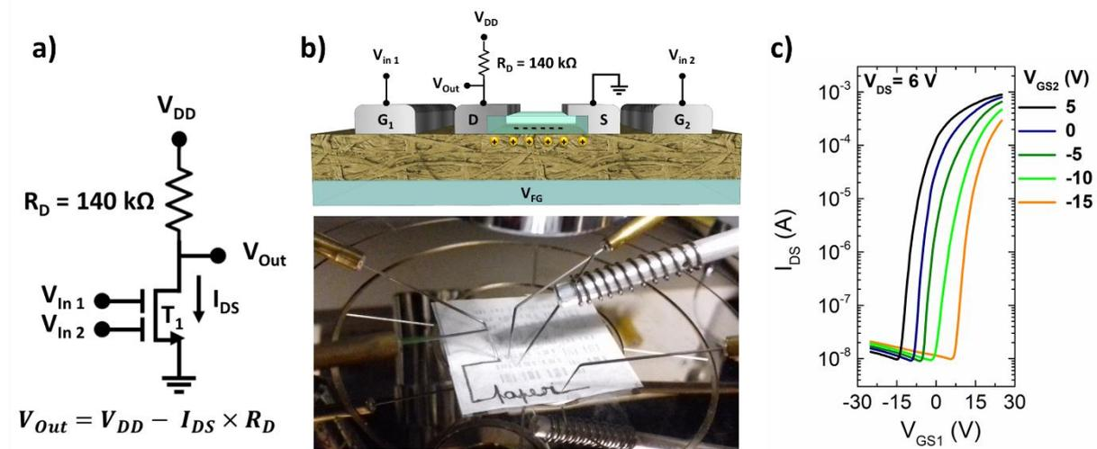
**Figure 1.** Universal logic gates: a) Circuit schematic, b) On-chip implementation, and c)  $I_{DS}$ - $V_{GS}$  transfer characteristics DG-FGFETs at  $V_{DS}=6$  V.
