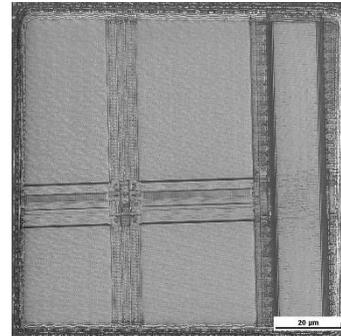
**Figure 2.** 500 eV SEM image of 100 × 100 μm window opened by Xe Plasma FIB-Gas Assisted Etching delayering. (Scale of 20 μm)
