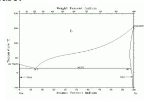
Fig. 2 Phase diagram of the Ga-In system [3].
