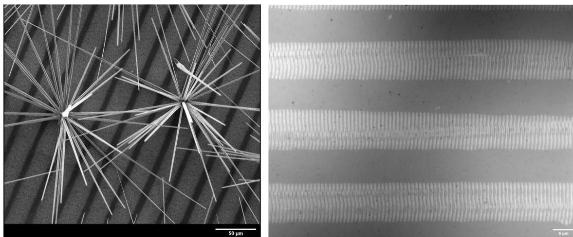
**Figure 1.** a) SEM image of the Zr doped ZnO structures growth on irradiated silicon substrate. b) Optical image of amorphous LIPSS in silicon  $\langle 100 \rangle$
