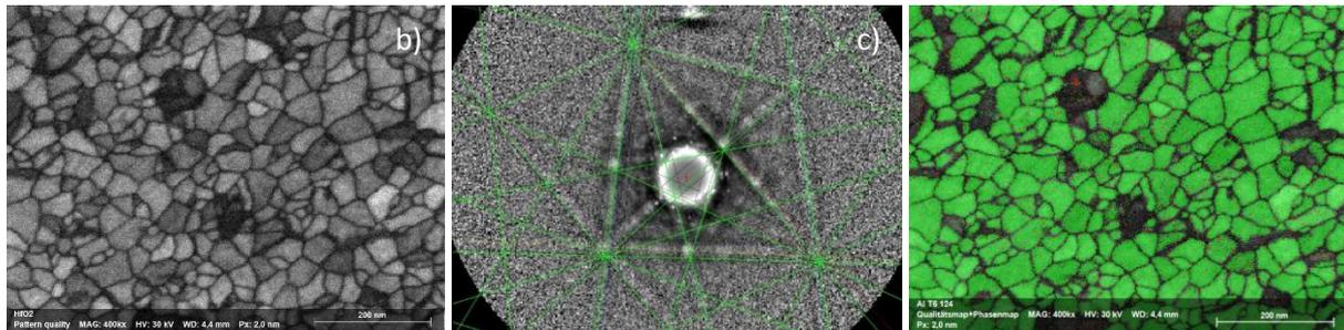
**Figure 1.** Phase identification of HfO<sub>2</sub> by TKD. From the EBSD pattern contrast of each point, a quality map (a) can be constructed. By comparing the EBSD patterns with simulated patterns from given phases (b), the phase can be identified and a phase map (c) can be constructed.
