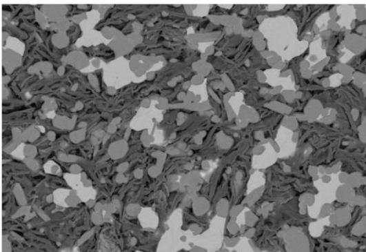
**Figure 1.** SEM image of Microstructure of the Ceramic-Carbon Composite
