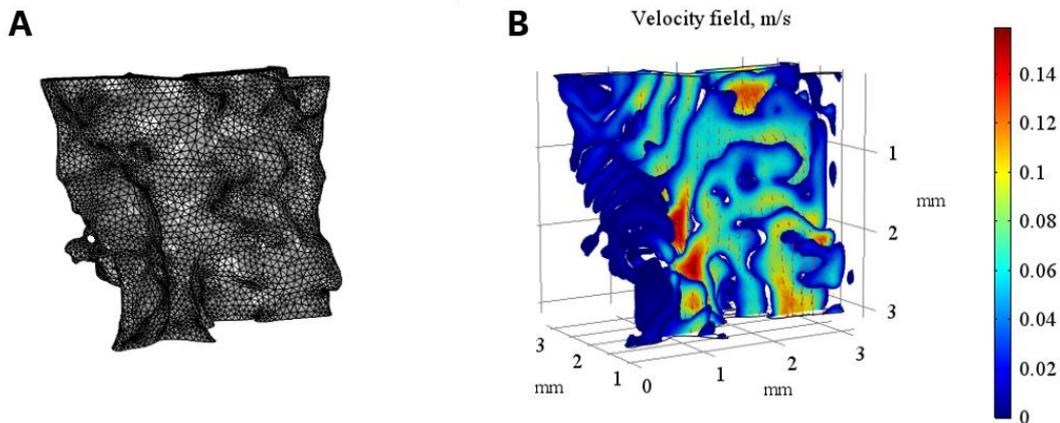
**Fig.1** A) 3D mesh created based on XCT observations. B) Result of the calculations – velocity field
