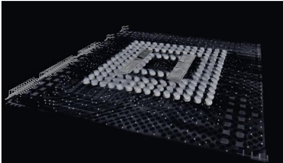
**Figure 1.** Reconstructed 3D CT image of Exynos 8995 chip.
