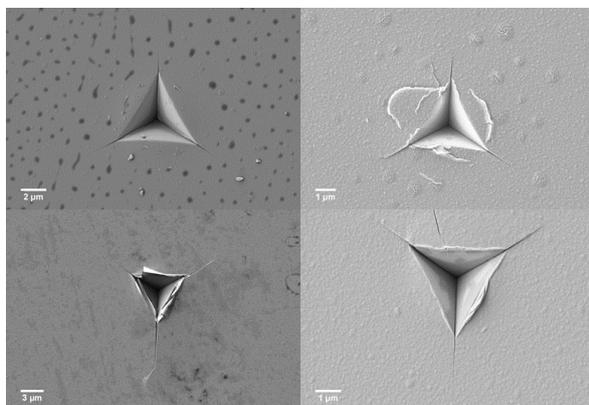
**Figure 1.** SEM micrographs of the indents on sample A (left) and sample B (right): upper images on fixed substrate, lower images with 100 % tensile surface stress applied.
