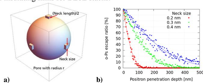
**Figure 1.** a) Pore model, to be repeated periodically in all three dimensions. b) Ps escape ratio for varying neck sizes
