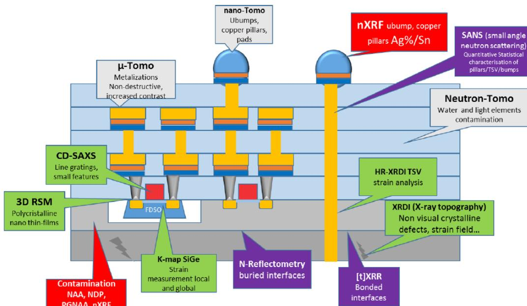
**Figure 1.** Scheme showing which neutron or synchrotron technique can be used to characterize a CMOS at every step of the process.
