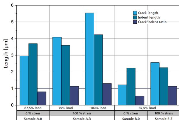
**Figure 2.** Crack length on sample A and B with varying stress and indentation loads.
