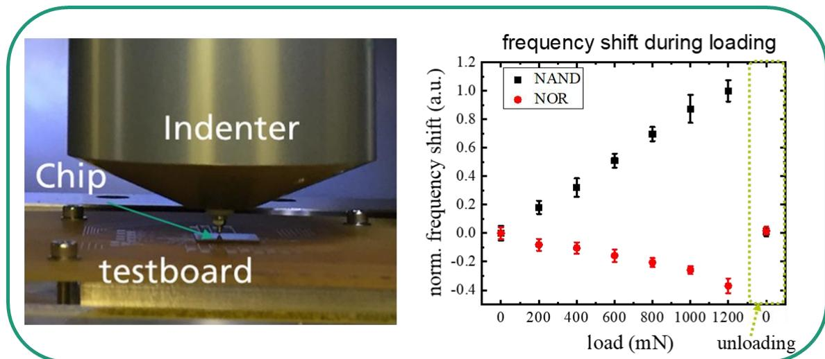
**Figure 1.** Experimental setup used for nanoindentation and obtained frequency shifts for NAND and NOR ring oscillator test structures.
