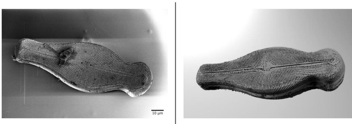
**Figure 1.** SEM image of diatom frustule and its respective FEM model. The FEM model was built based on reconstructed nano-XCT data. It consists of 21.6m tetrahedral, 1.2m hexahedral elements.
