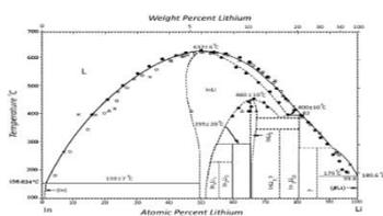
Fig. 3 Phase diagram of the In-Li system [4]
