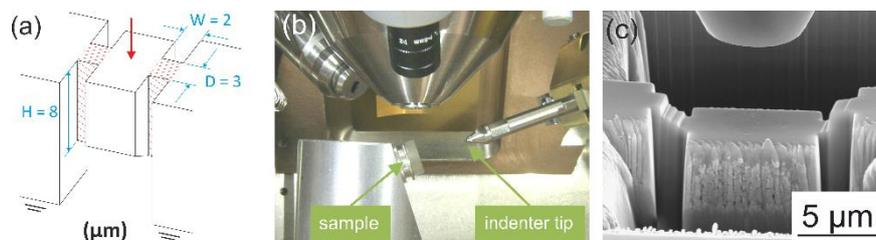
**Figure 1. Experimental setup:** (a) Microshear sample dimensions. (b) Test rig of in situ nanoindenter in a SEM chamber. (c) SEM micrograph after shear deformation of a FIB machined sample in single crystal Cu.
