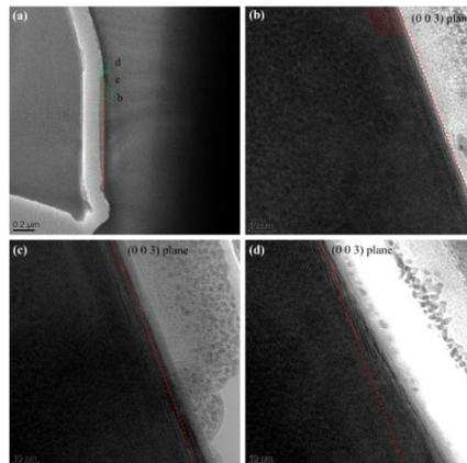
**Figure 1.** (a) Cleaved CaSi<sub>2</sub> lamella after in-situ test, (b), (c) and (d) HRTEM image of the area marked by the green square box.
