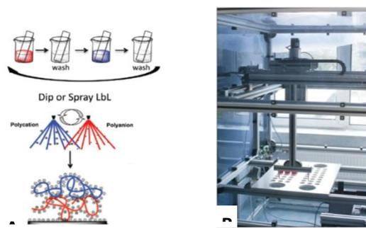
**Figure 1.** Polyelectrolyte Multilayer Film deposition process: A. Basics of the Layer by layer method [1,2], B. Automatic dipping machine, Laboratory of IMIM PAN
